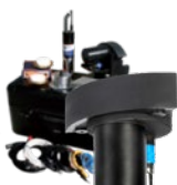
SEABED SPLMS (NORBIT WBMS + GPS RTK + INS + SVP + QINSY)
