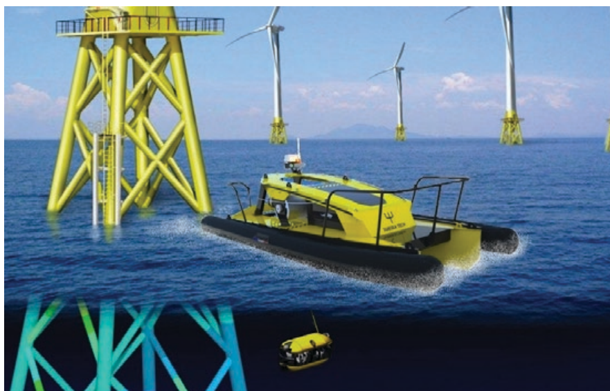
Multi-drone SeaCAT solution for inspection of MRE infrastructures
